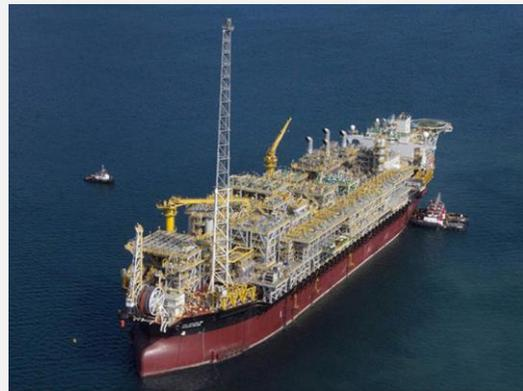
Figure 65 – Floating production, storage, and offloading (FPSO) unit<sup>77</sup>
